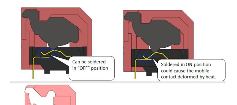
NDP new structure can be soldered either ON or
