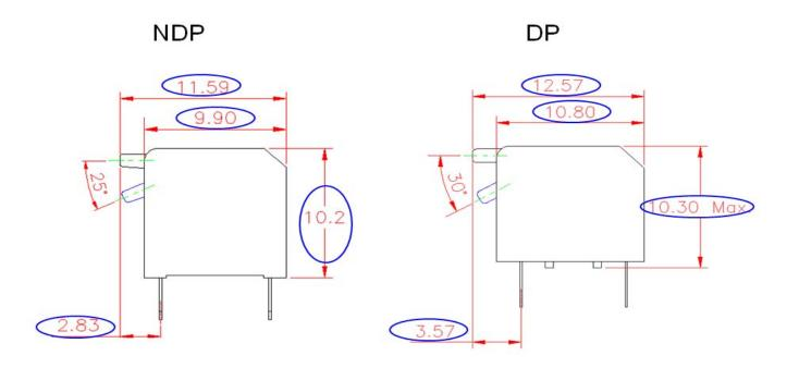
New Design Advantage: NDP can be solderable in "ON" or "OFF" position
